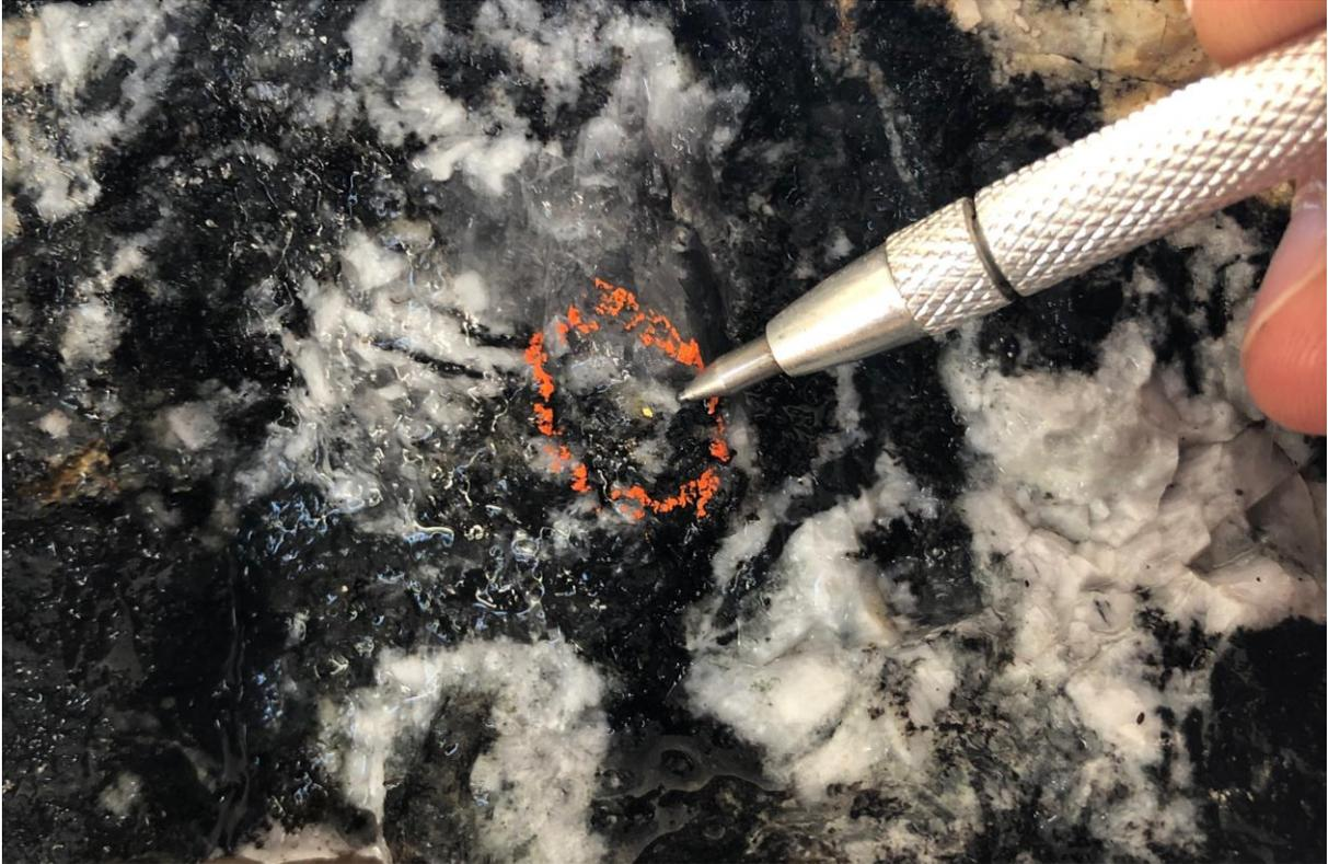
The visible gold in the picture above is from the A pit (westernmost) and is hosted by a pegmatitic quartz-albite-biotite vein. The outcrop that was blasted at this location returned several channel assays in the 1-3g/t Au range from a combination of blue quartz veins, and pegmatitic veins with arsenopyrite disseminations.
